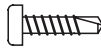
C0037 Screw Used for: Sill Drain Hole Cover, Header Interlock Plug and Condensation Drain
